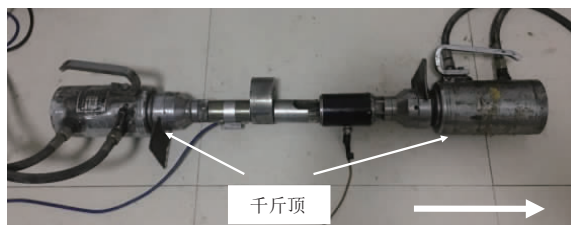
(c)步骤3:正向张拉,测试咬合力
