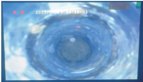
(c)注浆孔内窥镜检查
